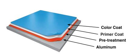
Alcotex finishes are applied in a reverse roller application process and are available in either a 2 or 3 coat finish. The 2 coat finish omits the clear coat required on a 3 coat finish. Both finishes will provide the same excellent performance required for architectural applications.
